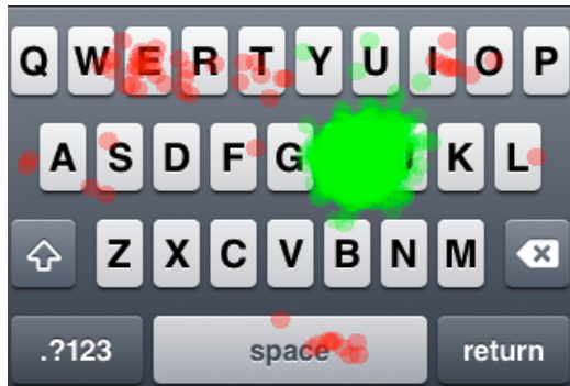
Figure 3. Tap filtering for letter “H”. Taps not on the intended key or its immediate neighbors are filtered out (in red).
