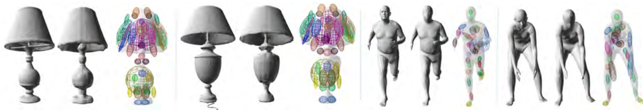
Figure 1. This paper introduces Local Deep Implicit Functions, a 3D shape representation that decomposes an input shape (mesh on left in every triplet) into a structured set of shape elements (colored ellipses on right) whose contributions to an implicit surface reconstruction (middle) are represented by latent vectors decoded by a deep network. Project video and website at ldif.cs.princeton.edu .
