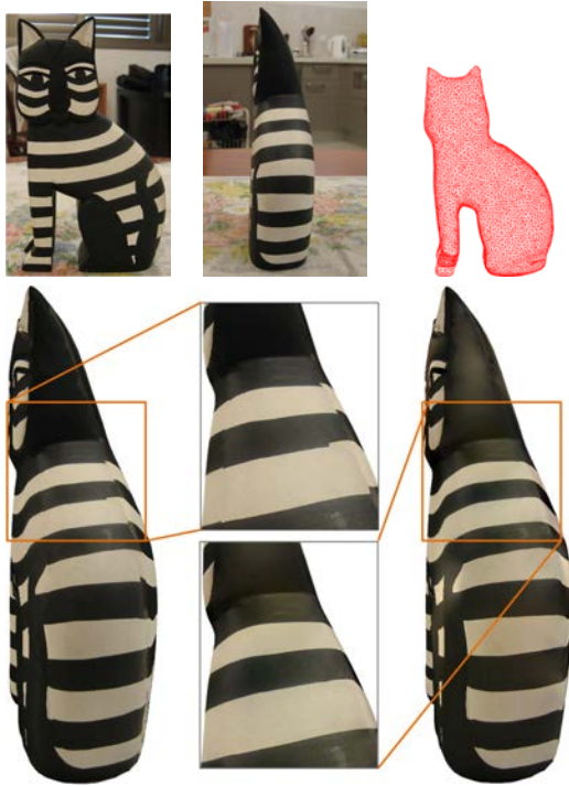
Figure 5: Example demonstrating the benefit of optimizing with translation shift vectors. Top row: two input images and reconstructed mesh. Bottom row: resulting texture montage without and with shift optimization.
