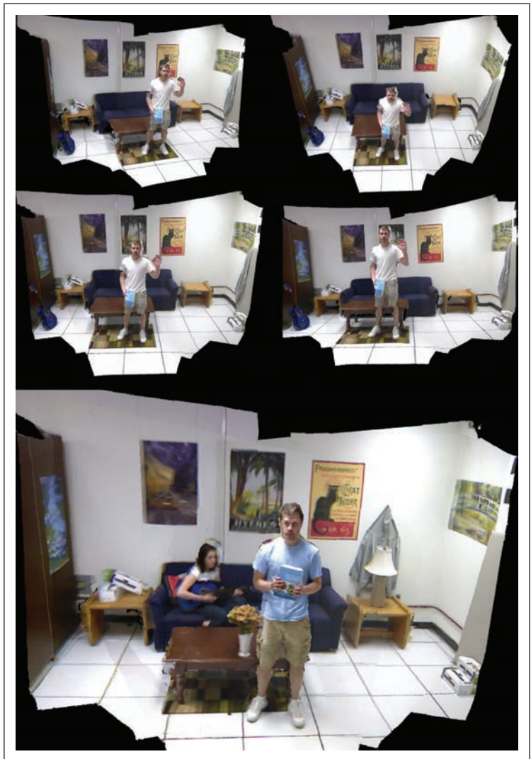
Figure 4. Virtual views of real-time 3D room reconstructions from 10 Kinect RGB-D cameras.
