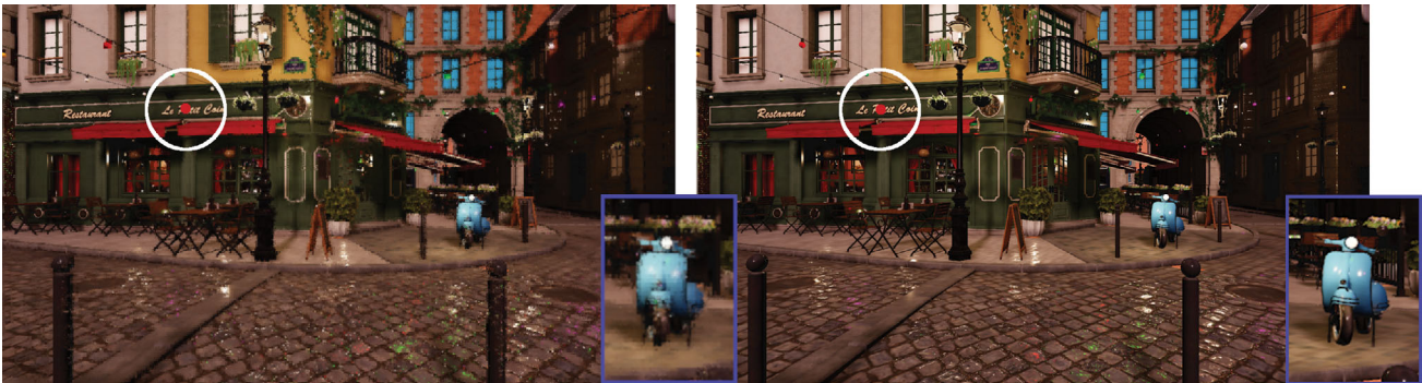
Figure 1: Our time-warped foveated rendering method produces visually plausible results (left, twice at 1280 \times 1440 pixels in 4.97ms on a RTX 2070) as compared to regular rendering (right, 7.81ms). While the fovea (which is tracked, indicated here in white) is rendered regularly, the periphery is reprojected, and thus less accurate, however without being noticeable to the observer's eye and in a temporally stable manner. Consequently, an image perceptually on par is computed with a speed-up of almost 1.6\times .
