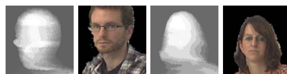
Figure 14 – Eye contact for virtual camera based on the estimated depth map and the rendered virtual view
