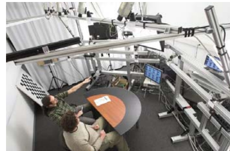
Figure 11 – top: Teleconferencing demonstrator concept including ceiling and side cameras for volumetric processing (top), experimental test mockup (bottom), possible camera arrangements (middle)
