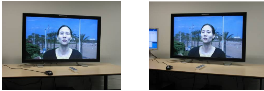
Figure 7 – Static image on the novel 2-view 3D prototype display, as seen: left) from the position of the left local participant, right) from the position of the right local participant.
