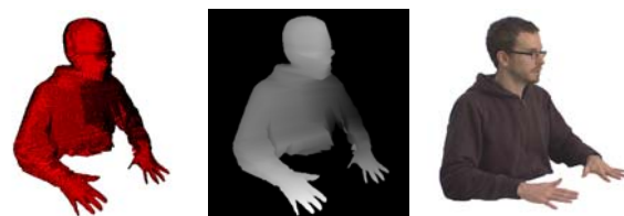
Figure 12 – Visual Hull result of a conferee, left: 3D model, middle: depth map representation, right: segmented input images
