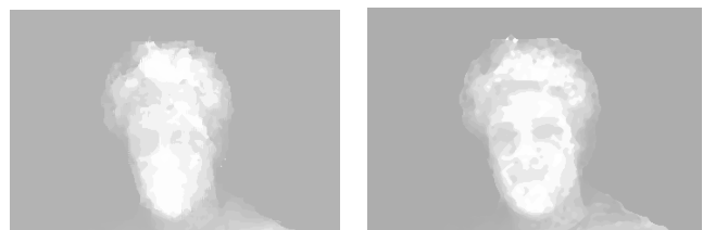
Figure 10 – Depth Layer: Small baseline (left), wide baseline refined (right)
