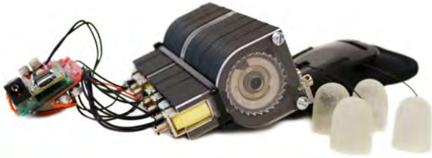
Figure 5. Example Wireality setup with seven haptic modules.
