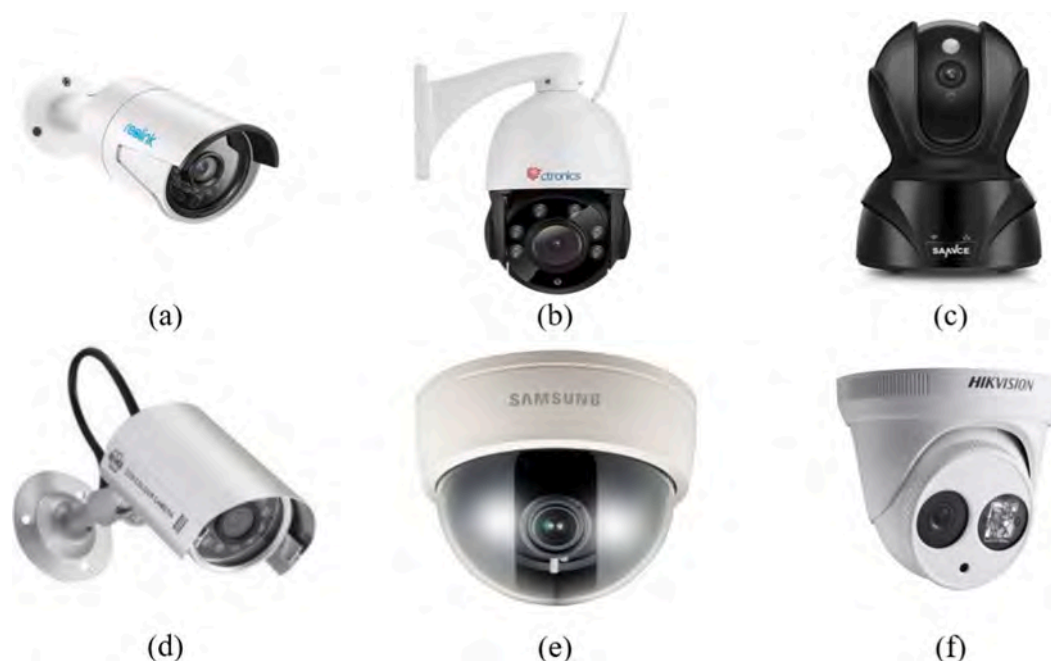
Fig. 8. Video surveillance cameras. (a) Fixed camera. (b) PTZ external camera. (c) PTZ internal camera. (d) Bullet camera. (e) Dome camera. (f) Turret camera.
