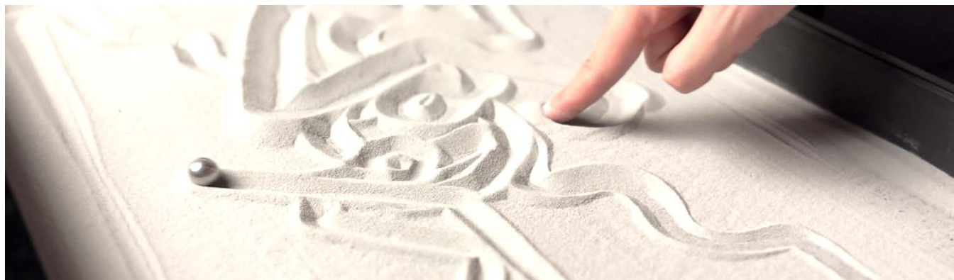
Figure 1: A user is drawing on the sand playground, and the metal ball draws synchronously.
