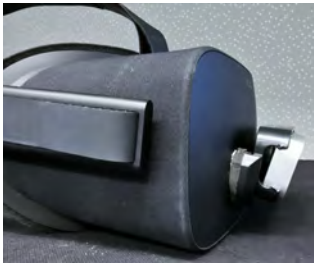
Figure 1: A Leap Motion Controller was attached to the front of the Oculus Rift at a 20° down angle to increase its field of view when the user's head is upright.
