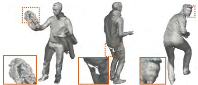
Figure 16: Current limitations of our system. From left to right: Noisy data when tracking is lost. Holes due to segmentation errors. Oversmoothing due to alignment errors.
