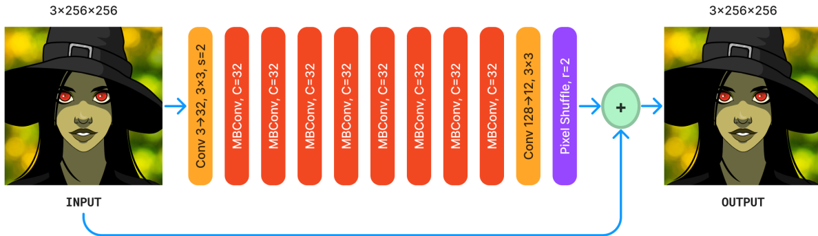
Fig. 1: Architecture of the residual network based on MBConv layers. This implementation depicts L = 8, C = 32 setup.
