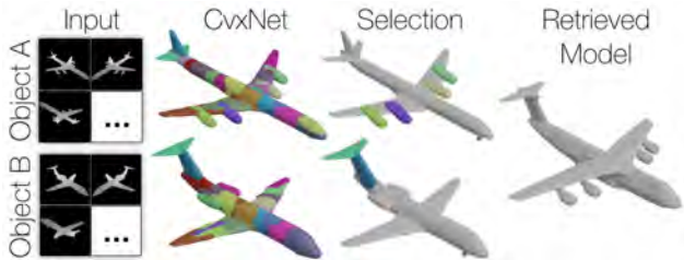
Figure 10. Part based retrieval – Two inputs (left) are first encoded into our CvxNet representation (middle-left), from which a user can select a subset of parts (middle-right). We then use the concatenated latent code as an (incomplete) geometric lookup function, and retrieve the closest decomposition in the training database (right).
