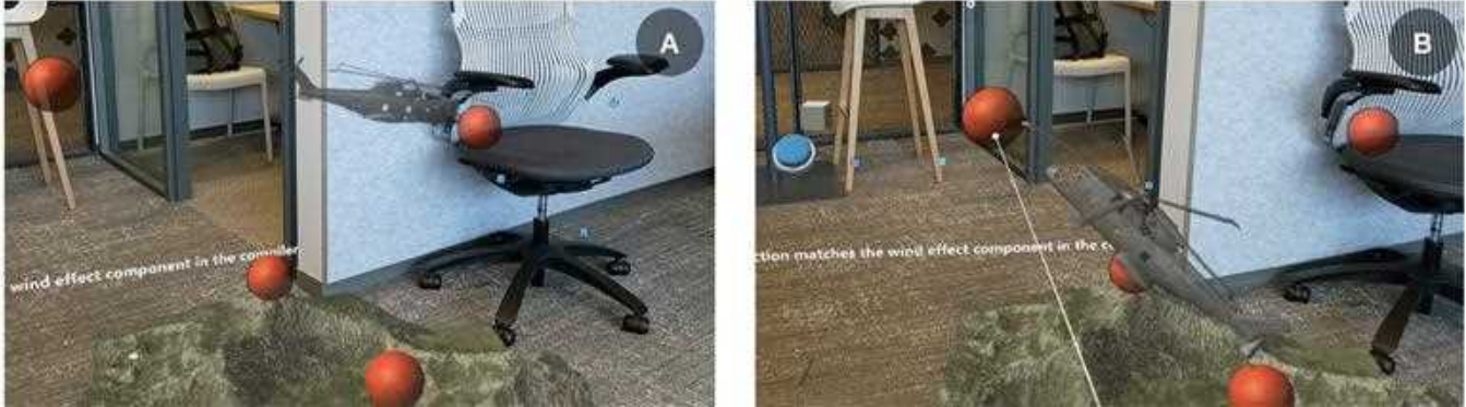
Figure 12: Simulated Rescue Plan. The HoloLens 2 displays the automated generation of a simulation of a rescue plan using our framework. The guide shows an interactable 3D terrain, helicopter, and simulated wind, allowing rescue workers to visualize the flight path under different weather conditions.
