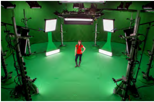
Figure 3: Typical stage setup. RGB and IR cameras and unstructured static IR laser light sources surround the capture volume.
