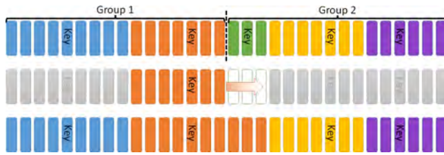
Figure 9: To parallelize mesh tracking, we first partition frames into groups and process groups in parallel using Algorithm 1. To improve the possibly suboptimal result near group boundaries, we join the frames covered by the boundary keyframes (orange and green) and reapply Algorithm 1. The algorithm often completes using a single keyframe (bottom), thus effectively removing a keyframe (green).
