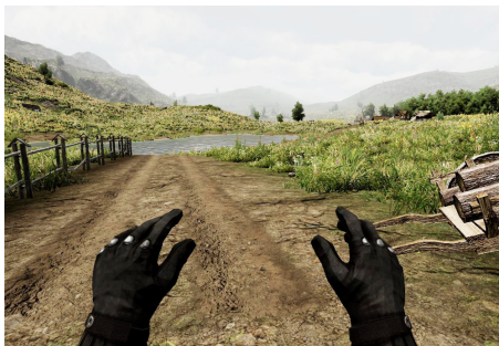
Figure 1: Navigation Technique: Start in first-person (1), grow to third-person perspective and set a navigation target (2), wait for the avatar to walk there and switch back to first-person (3).
