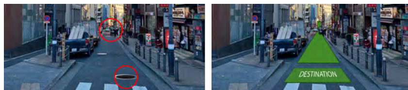
Fig. 1. Digital overlays can obfuscate critical information, such as manholes or the view ahead [10].
