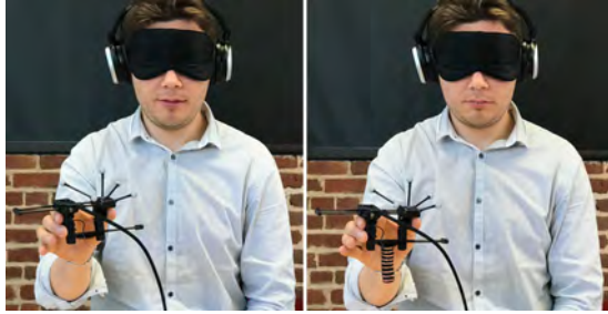
Figure 11. Virtual force measuring experiment setup. Right: Device with added physical weights.
