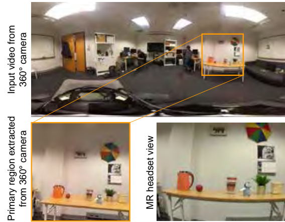
Fig. 4. One frame of the 360° input video (top), extracted primary region (bottom left) used for processing, and MR headset view (bottom right) used for alignment.
