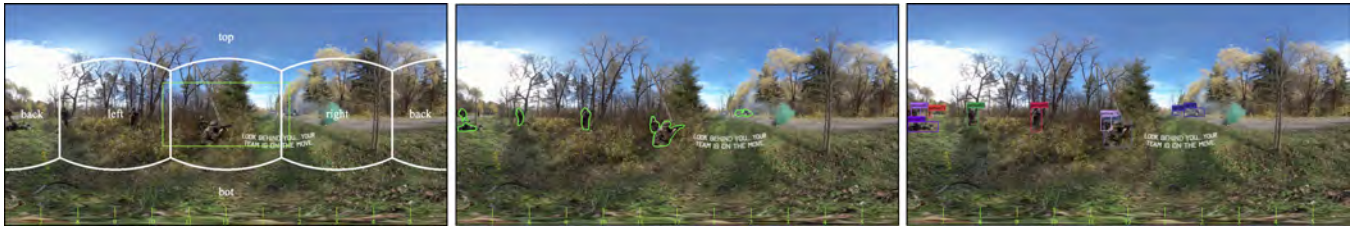
Figure 6: OmniScribe visual overlays: (left) section division outlines the top, bottom, front, back, left, and right. (middle) The visual saliency overlay. (right) The object recognition and tracking overlay.
