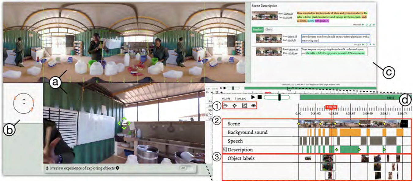
Figure 3: Overview of the OmniScribe description authoring interface. (a) The augmented equirectangular view with clock meter (top) and NFOV (bottom). (b) Content map presenting dynamic objects and viewing angle. (c) Description authoring panel for authoring standard AD, as well as scene and object descriptions. (d) Timeline panel (zoomed-in view): 1) toggles for selecting video files, section division, object tracking, and saliency overlays (left-right); 2) timelines for the scene, background sound, speech, and description. The yellow diamonds marked in the scene layer represent the created scene descriptions. The green diamonds marked in the description layer represent the extended descriptions; and 3) the created object descriptions are visualized by object thumbnails.
