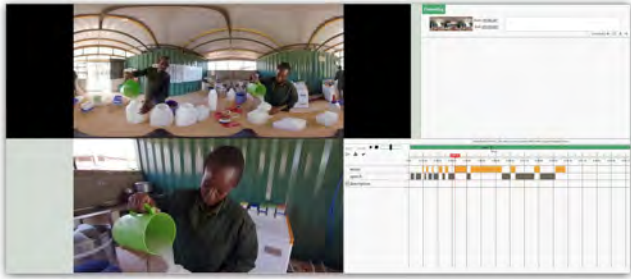
Figure 9: Interface for our Baseline condition, which includes the equirectangular view and NFOV (similar to Final Cut Pro), the description panel, and the timeline panel with visualized audio profiles of the video.
