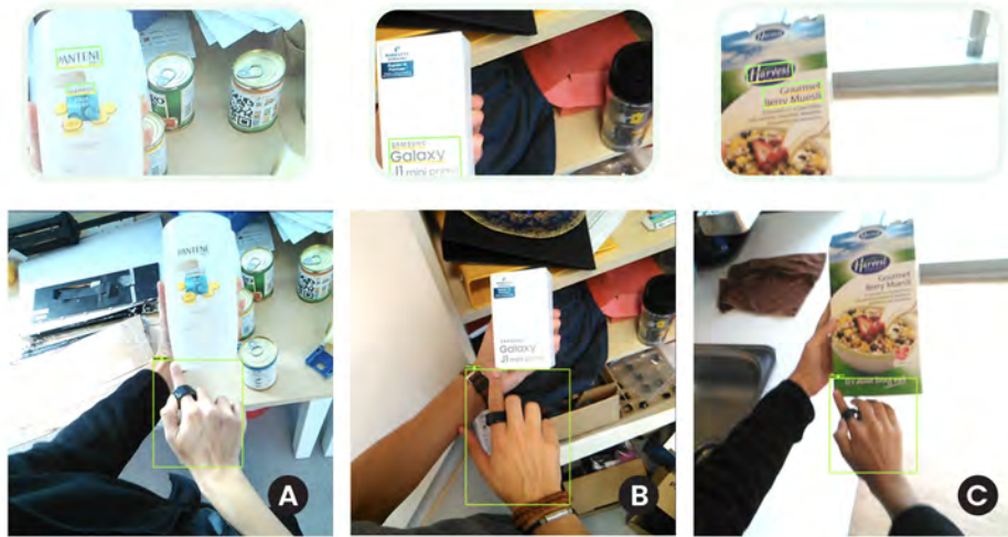
Fig. 7. Bottom row: original images extracted from the camera after identifying the gesture. Top row: cropped images after extracting the Region of interest.
