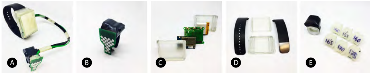
Fig. 2. Prototype components: (A) Wristband connected to the ring (B) Ring with touch-pad (C) Intel Edison, PCB, battery, and wristband 3D-printed casing (D) Casing and straps, and (E) Ring and 3D-printed fittings of different sizes
