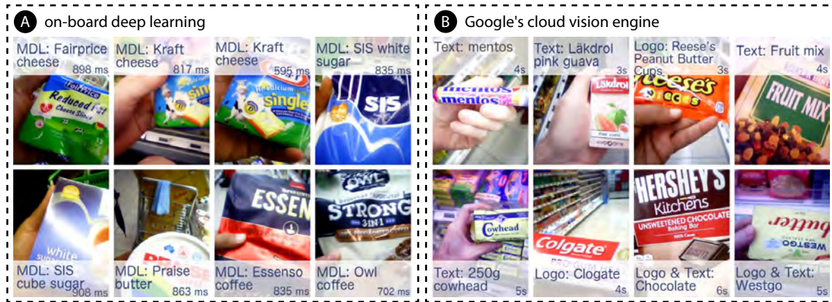
Fig. 3. Successfully recognized images during our field study: A) using our on-board deep learning, yielding low recognition delays <1s , B) using the Google cloud vision engine for untrained products yielded significantly higher delays >3s .
