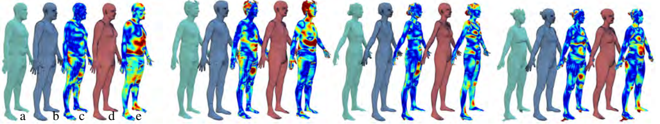
Figure 6: Shape evaluation for Seq. 1. Comparison between ground-truth scans (a) in green, our estimated models (b) in blue, and BodySnap models (d) in red for 4 subjects. Heat maps (c) and (e) beside each model show the scan-to-model registration error for our method and BodySnap, respectively (blue means 0mm, red means \geq 1 cm).
