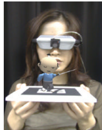
Figure 1: The user interacts with 3D virtual objects by manipulating a tangible object; such as a simple paper card.
