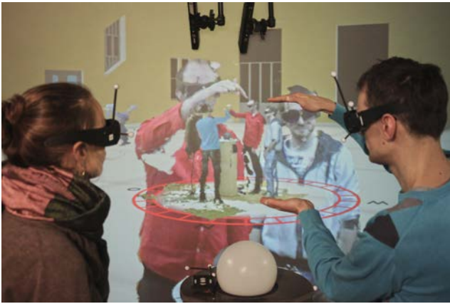
Fig. 9. Two groups of users are standing across from each other and around the overlapping Spheron input devices. They zoomed into the WIM to the location where they are currently located in the city model. Here they can see video-avatar representations of themselves.
