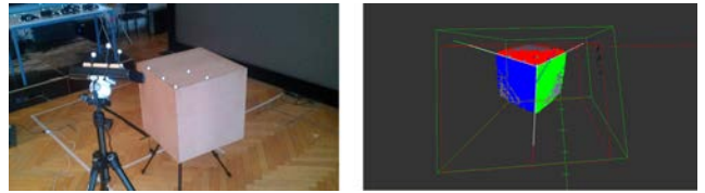
Fig. 5. Left: The calibration box with markers attached and a Kinect that has to be registered. The three sides of the box are exactly orthogonal. Right: The three sides of the box are detected in the depth image. The deviation between the computed coordinate system (colored axes) and its orthonormal form (white axes) is below 0.3 degree per axis.
