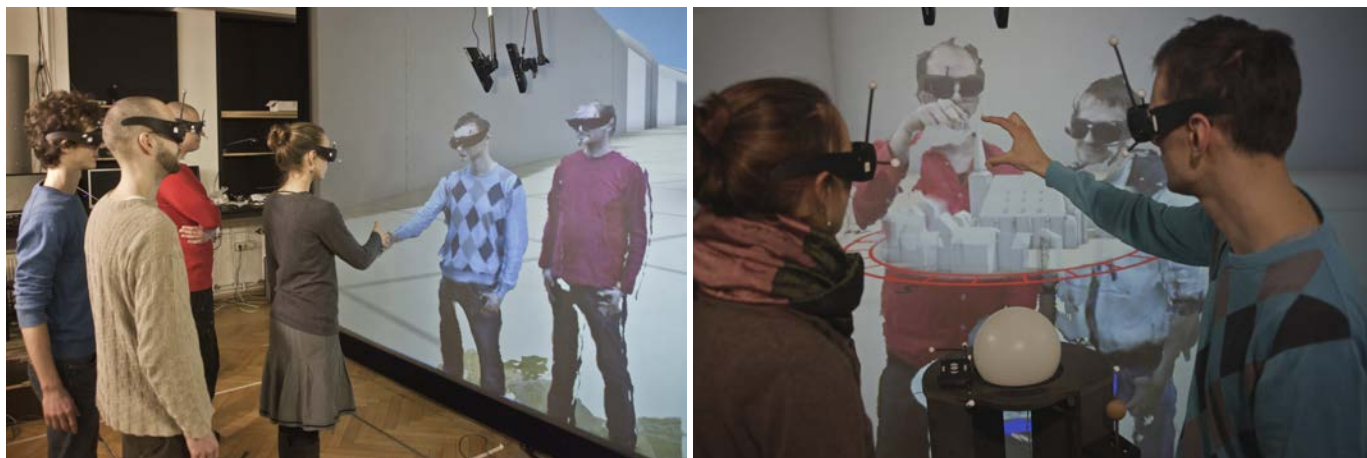
Fig. 1. Two groups of users meet virtually while being surrounded by a virtual city. On the left the local users greet the life-size 3D representations of the remote users. On the right the two groups discuss the tower of a church in a WIM by pointing and gesturing.
