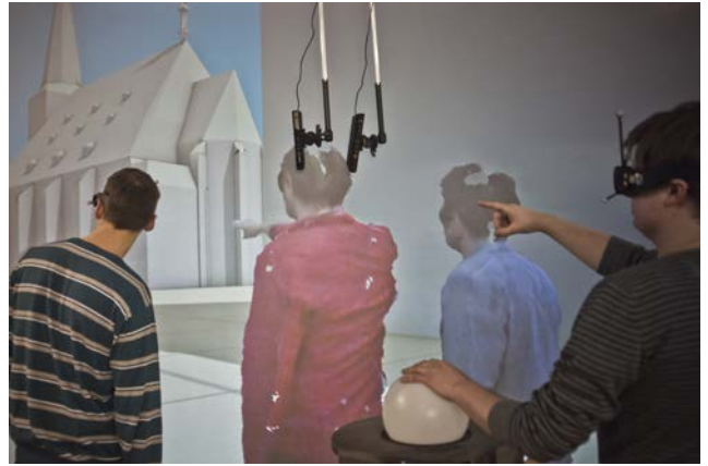
Fig. 10. The two groups stand next to each other. The user on the right side is standing behind the remote users and thus he can see their virtual representations from behind.
