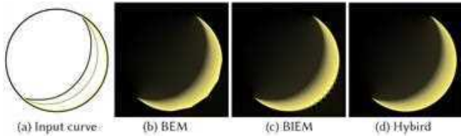
Fig. 4. Result comparisons between BEM, BIEM, and our Hybrid method. BEM suffers from visible polyline, and BIEM shows dotted-looking artifacts near the boundary, whereas our method is free from both problems.
