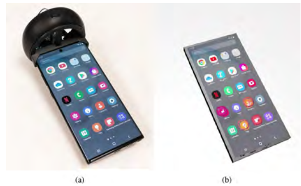
Fig. 4. (a) The tracked phone in reality. (b) The real-time mirrored and textured virtual proxy phone.
