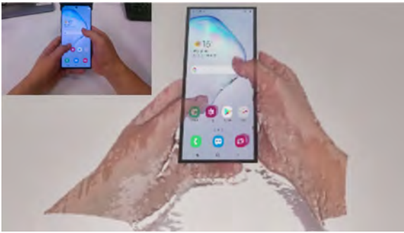
Fig. 1. A virtual smartphone with real-time screen updating is reproduced in a VR environment. The user can see his/her own hands and touch the virtual phone with tangible feedback.
