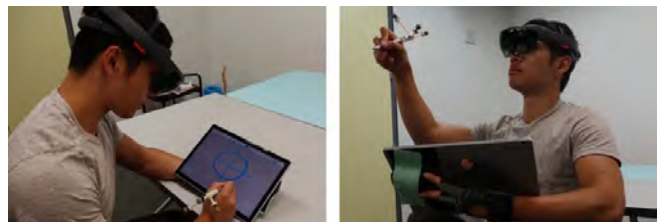
Figure 6. Setup: the user puts on the HoloLens and draws with a motion-tracked stylus, on a tablet (left), or mid-air (right) using a mouse affixed to the back of the tablet.
