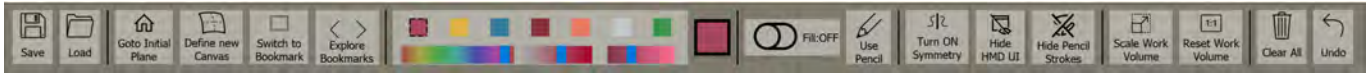
Figure 8. 2D UI toolbar. (left to right) save/load, initial canvas , create canvas , explore and select bookmarks, color tools (palette, HSV sliders, indicator), fill, pencil/ink toggle, symmetry plane, UI and pencil toggles, workspace scaling and reset, clear all and undo stroke. Buttons are shown only if currently useful. For example, selecting the pencil hides color tools. Icons © icons8.com. Used under CC BY-ND 3.0.
