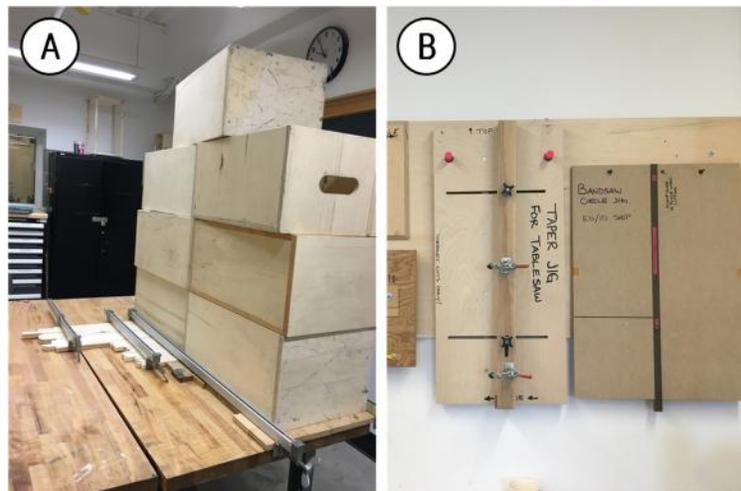
**Figure 6. Specialized accessories that were created to overcome limitations with workshop tools: (A) a series of milk crates acting as weights to help with the lamination of a series of wood strips in the First-Year Teaching Shop and (B) a taper jig for use with a table saw was used in the Industrial Design Studio because a commercial version could not be found.**
