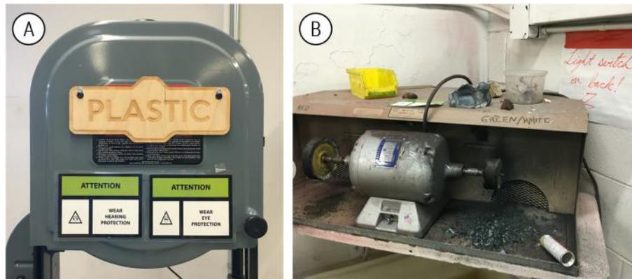
**Figure 9. Examples of the “documentation” and assistance that could be found in the (A) Industrial Design Shop and (B) Wax Studio. The ‘Plastic’ sign informed participants that the bandsaw could only be used for plastic but did not provide any other instructions. The only instructions for the grinder were the ‘red’ and ‘green/white’ labels on the outer casing and the hand-written sign indicating the location of the light switch.**
