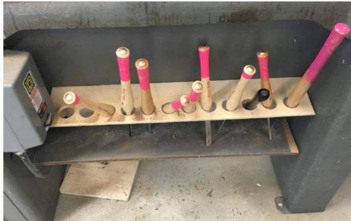
**Figure 4. Chisels located in the base of a lathe enabled easy access to them.**
