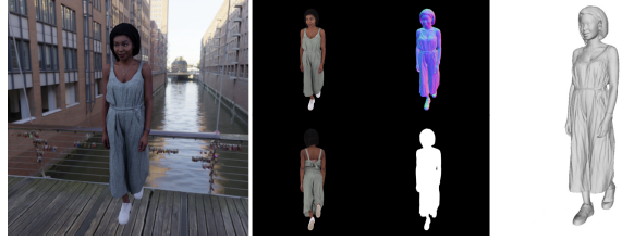
Figure 3. A sample from our dataset. From left to right: rendered, shaded image on HDRI background; front and back albedo images; normal and an alpha map, and 3D mesh used for sampling.
