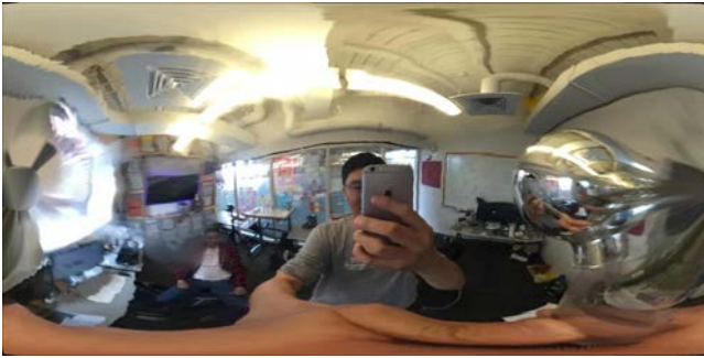
Figure 2. Equirectangular projection of image from sphere.
