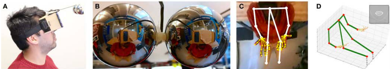
Figure 1. A) MeCap accessory attached to Google Cardboard. B) View of two mirrored spheres as seen by a smartphone's rear-facing camera. C) Unwrapped, virtual view looking down at a user's body, with hand and body keypoints overlaid. D) The 3D position of keypoints can be estimated through reverse raycasting stereo correspondence.
